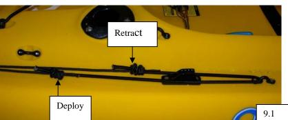
2. With rudder blade in up position, begin first knot by taking the retract line and looping over the bungee line two times, from left to right in a crisscross pattern. See 9.2.
