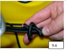
the excess rope and bungee leaving about an inch. Use a lighter or other heat source to melt the ends of the
