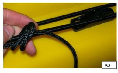
rope. Use hot glue to seal the ends of the bungee.
